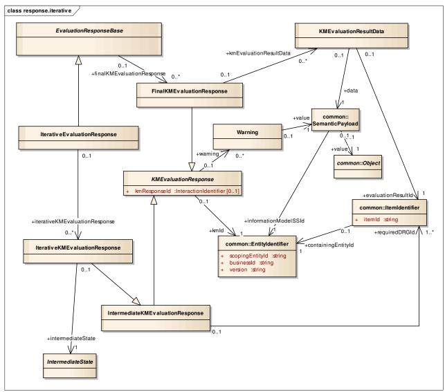
Figure 6.25. Model for Iterative Evaluation Response.
