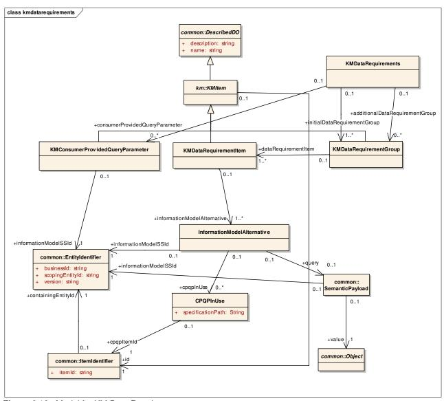
Figure 6.16. Model for KM Data Requirements.
