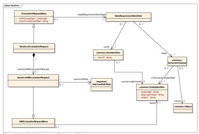
Figure 6.23. Model for Iterative Evaluation Request.
