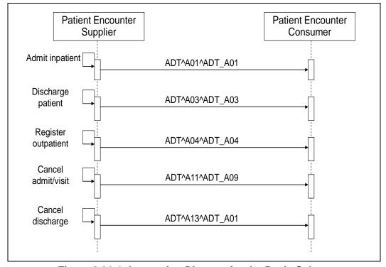
Figure 3.31-1: Interaction Diagram for the Basic Subset
