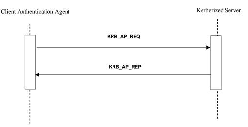
Figure 3.4-1 Kerberized Communications
