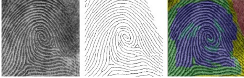
Figure 40: Examples of fingerprint, skeletonized representation, and overlay of original / skeleton / quality map
